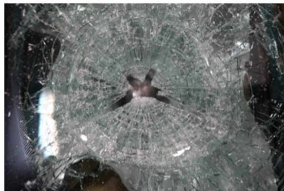
Fig. 2. Unsuccessful (NOK) test result (Nováček, 2024)
