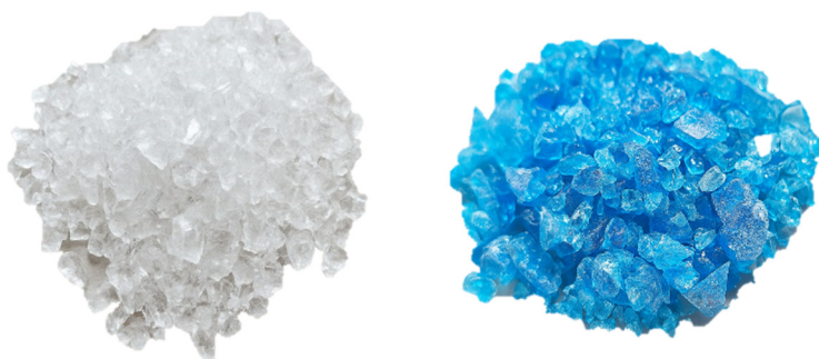
Fig. 1. Waste glass used for testing before sieving ( own research )
