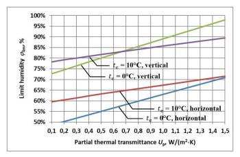
Fig. 2. Dependence of air humidity, at which water vapor condensation on the envelope surface is possible, on its insulation, for  $\varepsilon = 0.85$  (own research)
