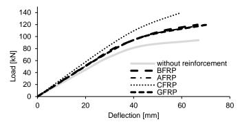
Fig. 3. Displacement-force plot for analyzed beams (own study)
