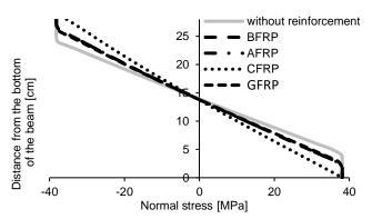
Fig. 4. The plot of normal stresses in timber for the analyzed beams (own study)
