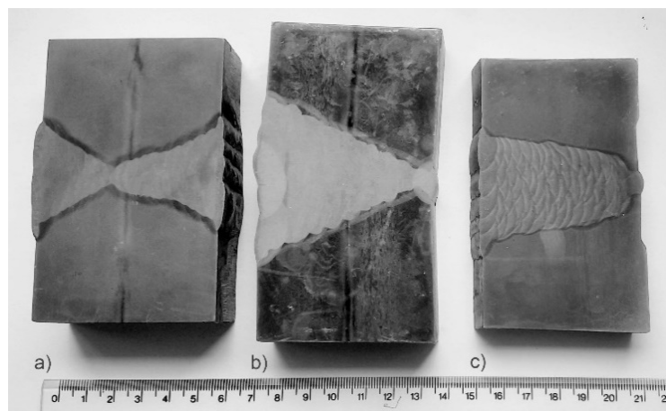
Fig. 3. Butt welds: a) double-V (X), b) V, c) single-U ( own research )
