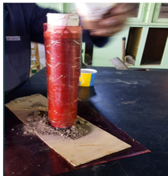
Fig. 3. Resin added in external mold ( own photo )
