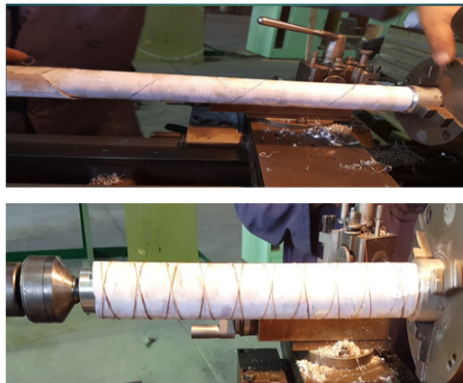
Fig. 2. Delimited angle and winding fiber ( own photo )
