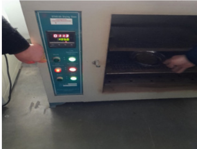
Fig. 1. Process of drying materials to constant weight ( own research )
